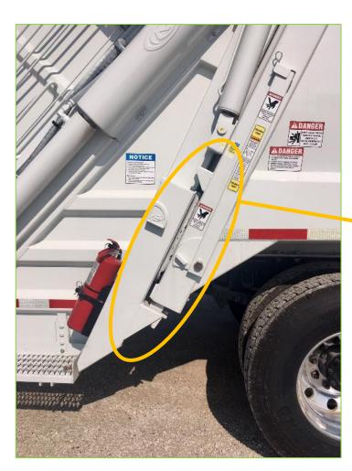
In-cab air controls; keep operator in cab with automatic tailgate locks
