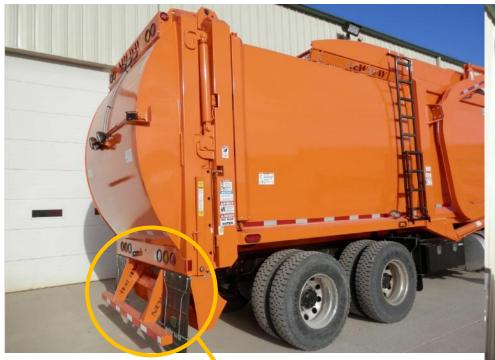
Tailgate drip pans: Redundant spill protection
