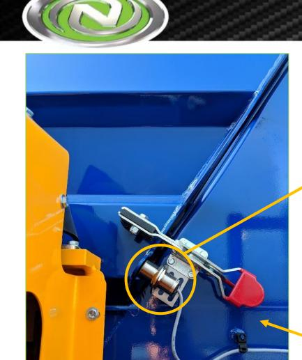
Proximity Switches: Indicate to operator components out of position
