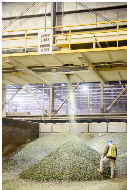
After SMI receives glass from MRFs it is further cleaned for end-markets. Clean emerald (green) glass at an SMI glass processing plant.
