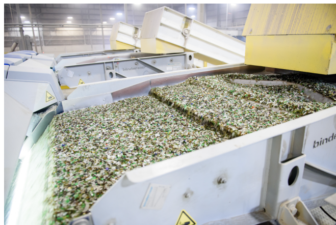
Glass optical sorting machine removes fines at SMI plant.
