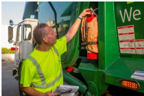
Inspecting fire extinguishers
