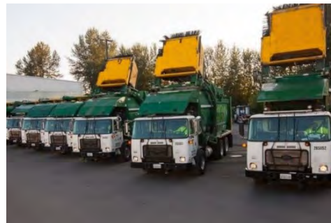
Testing hydraulic lifts and buckets
