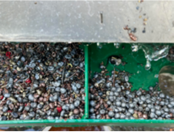
Figure 1 - Granulated copper, aluminum, brass, zinc, mixed alloys, stainless steel, and other metals recovered from landfill material are size-reduced using a hammermill and then density-sorted on a wet shaker table to separate metallic from non-metallic fractions.
