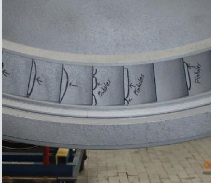
Stage 9 LH Pinholes in Partitions
