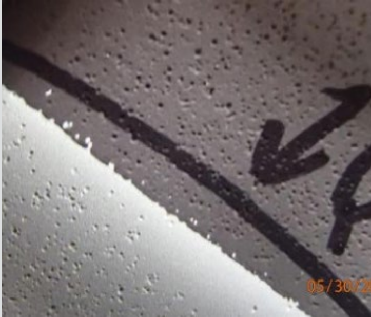
Stage 10 LH Pinhole in Partition Trailing Edge
