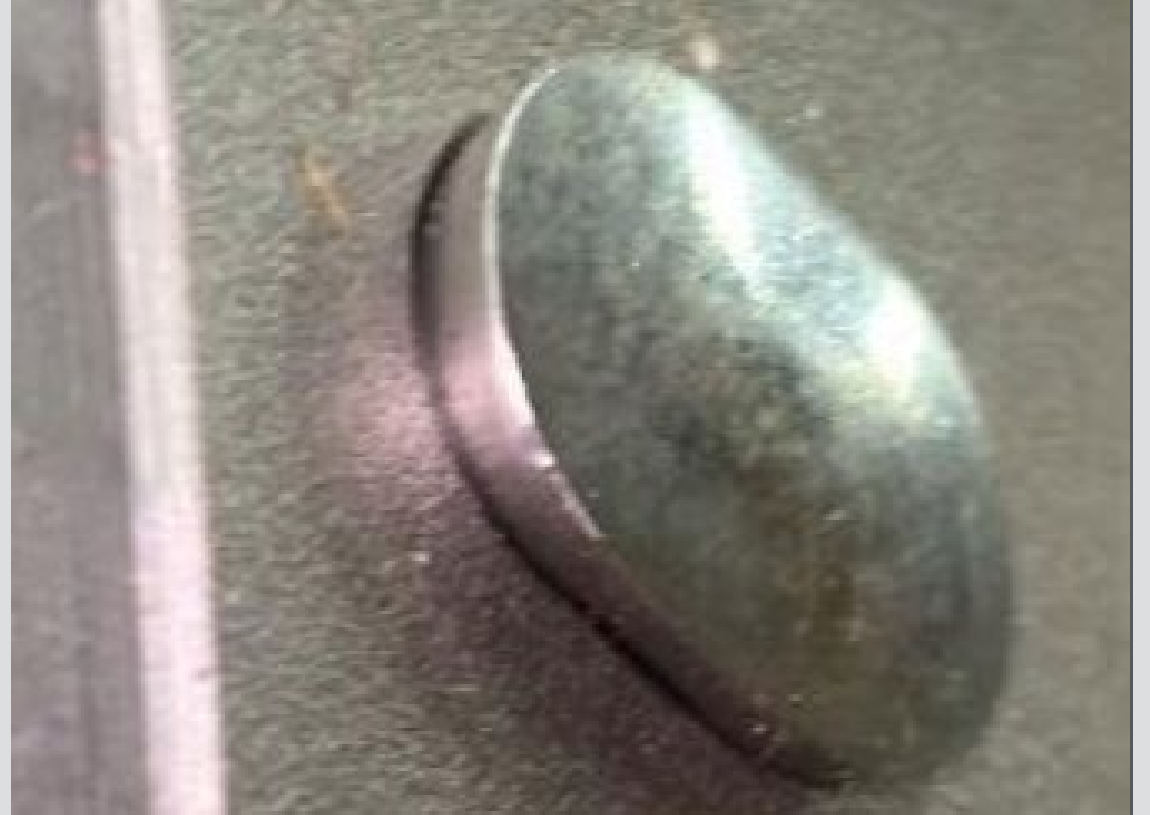
Stage 11 (New) Tenons – High, Chamfer Visible; several blade edges dented
